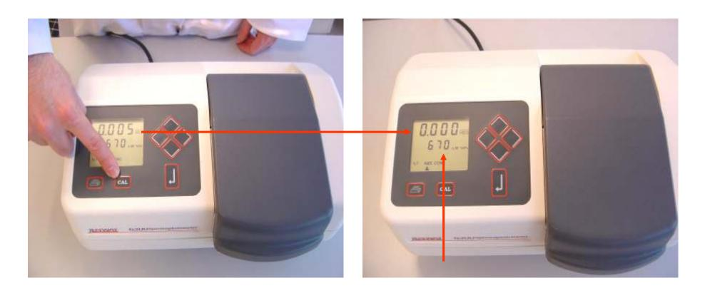
ZERO-CALIBRATE THE INSTRUMENT AT A WAVELENGTH OF 670 NM
