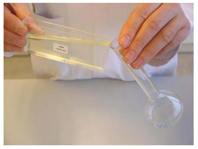
POUR THE 25 ML ALGAL SUSPENSION FROM THE ALGAL STOCK CELL INTO A 100 ML FLASK
