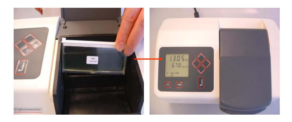
PUT THE ALGAL STOCK CELL IN THE SPECTROPHOTOMETER AND READ THE OPTICAL DENSITY (**OD1**) AFTER 10 SECONDS
