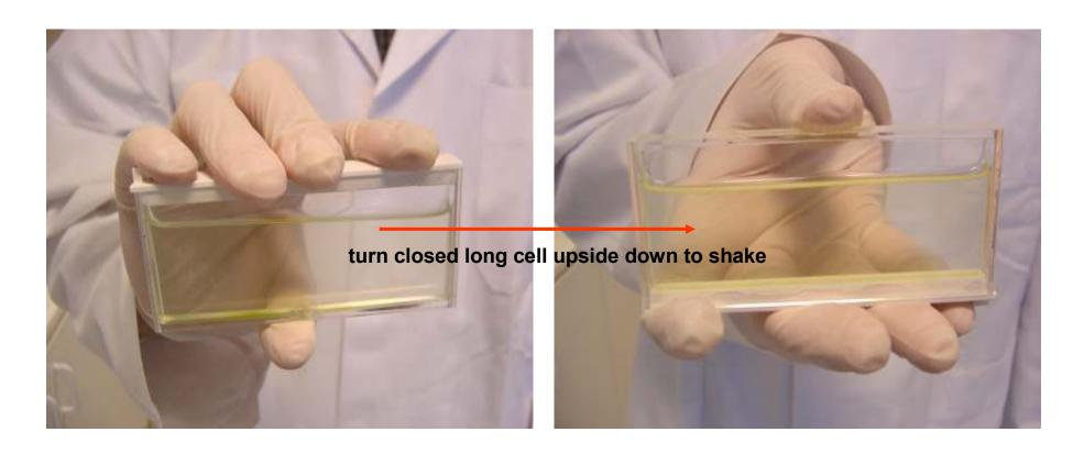
IMMEDIATELY BEFORE MEASURING THE **OD** IN A LONG CELL, CLOSE THE CELL, TURN IT UPSIDE DOWN AND SHAKE GENTLY TO RESUSPEND THE ALGAE EVENLY
