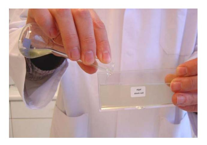
TRANSFER THE 25 ML ALGAL SUSPENSION INTO THE ALGAL STOCK CELL
