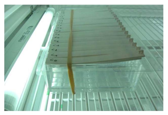
INCUBATE THE HOLDING TRAY WITH THE LONG CELLS FOR 72h IN AN INCUBATOR AT 23°C  $\pm$  2 °C, WITH CONTINUOUS ILLUMINATION:
