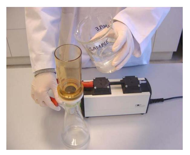
TO ELIMINATE TURBIDITY, SAMPLES MUST BE FILTERED BEFORE TESTING (e.g. over a membrane filter of 0.45  $\mu$ m),
