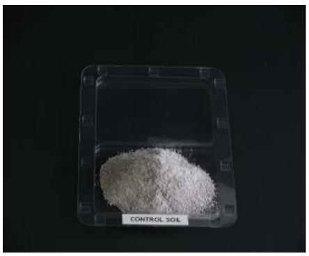
POUR THE CONTENTS OF ONE BAG WITH REFERENCE SOIL (90 ML) IN THE LOWER COMPARTMENT OF A TEST PLATE
