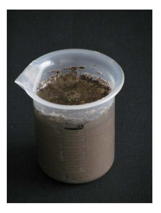
WAIT FOR THE SOIL/WATER MIXTURE TO REACH EQUILIBRUM, LEADING TO A WATER SATURATED SOIL PHASE AND A LAYER OF WATER ON TOP
