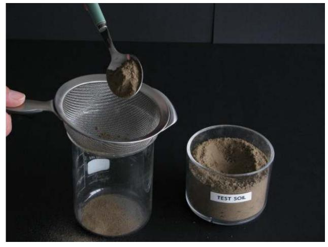
SIEVE AIR-DRIED SOIL THROUGH A SIEVE WITH A 2MM MESH TO ELIMINATE ALL COARSE MATERIAL
