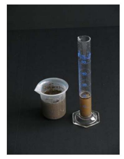
WAIT FOR A FEW MINUTES AND POUR AGAIN THE WATER ON TOP OF THE SOIL IN THE GRADUATED CYLINDER
