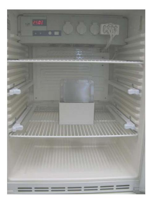
PUT THE CARDBOARD HOLDERS WITH THE TEST PLATES IN THE INCUBATOR AND INCUBATE AT 25° C, FOR 3 DAYS, IN DARKNESS
