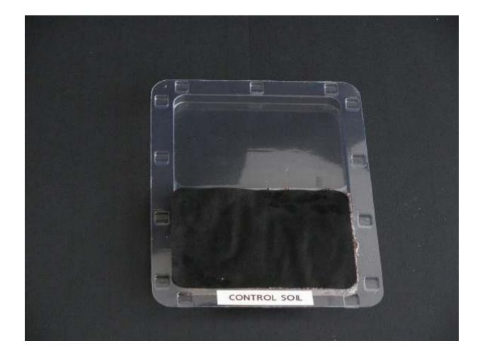
PUT A BLACK FILTER ON TOP OF THE HYDRATED (CONTROL AND TEST) SOILS IN ALL THE TEST PLATES AND WAIT UNTIL THE FILTER IS COMPLETELY WET
