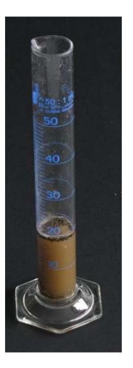
CALCULATE THE VOLUME OF WATER (Vsat) NEEDED FOR COMPLETE HYDRATATION OF THE TEST SOIL.
