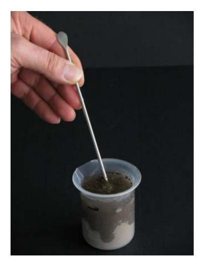
MIX THE WATER THOROUGHLY WITH THE SOIL TILL THE SOIL IS COMPLETELY WATER SATURATED
