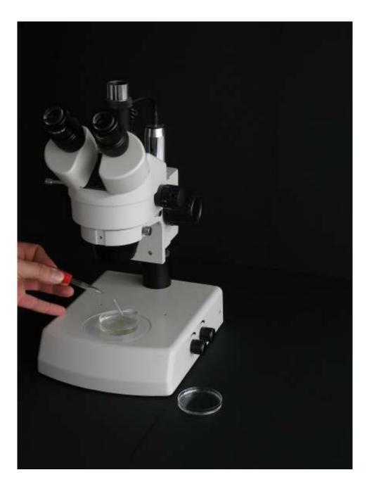
TRANSFER WITH THE GLASS MICROPIPETTE A NUMBER OF OSTRACOD NEONATES FROM THE HATCHING PETRI DISH INTO THE LID OF THIS DISH
