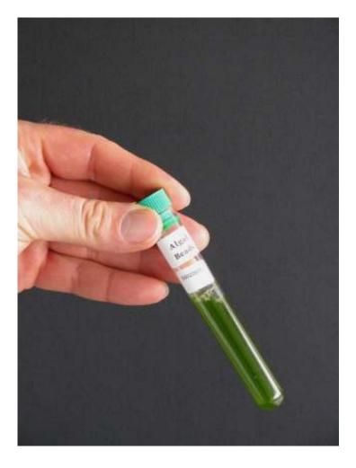
ADD 10 ML DISTILLED WATER TO THE TUBE WITH THE ALGAL PELLET CAP AND SHAKE THE TUBE TO RESUSPEND THE ALGAE
