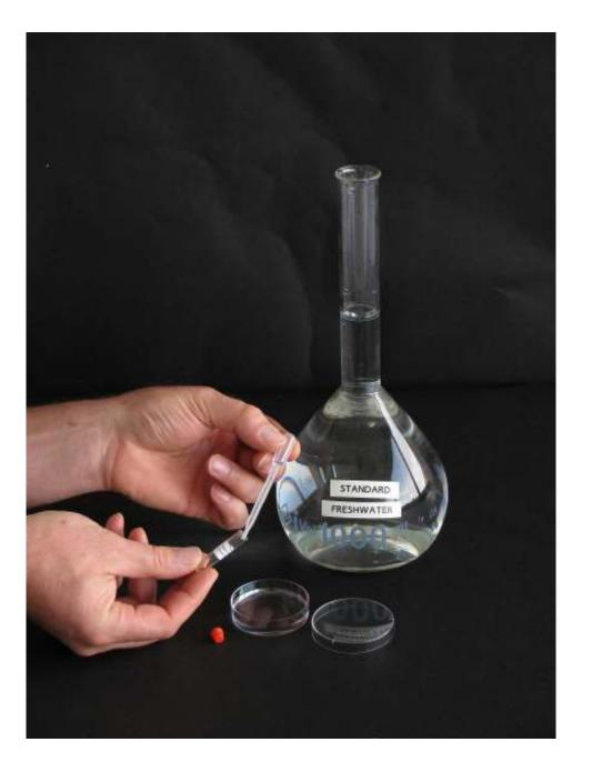
TO ENSURE THE TRANSFER OF ALL THE CYSTS, THE VIAL SHOULD BE RINSED TWICE WITH 1 ML STANDARD FRESHWATER
