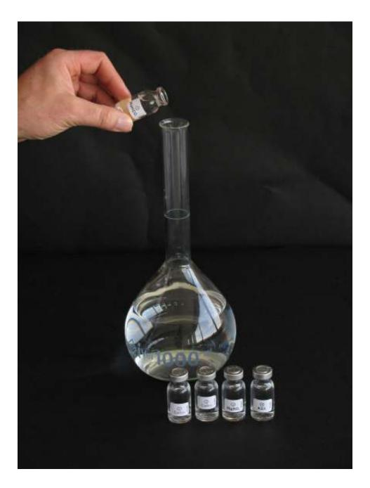
POUR THE 5 VIALS WITH CONCENTRATED SALT SOLUTIONS IN <u>+</u> 800 ML DISTILLED WATER, IN THE 1 LITER VOLUMETRIC FLASK
