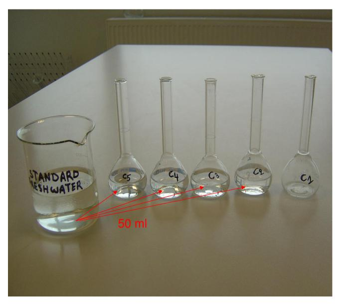
TRANSFER 50 ML STANDARD FRESHWATER INTO FLASKS C2, C3, C4 AND C5
