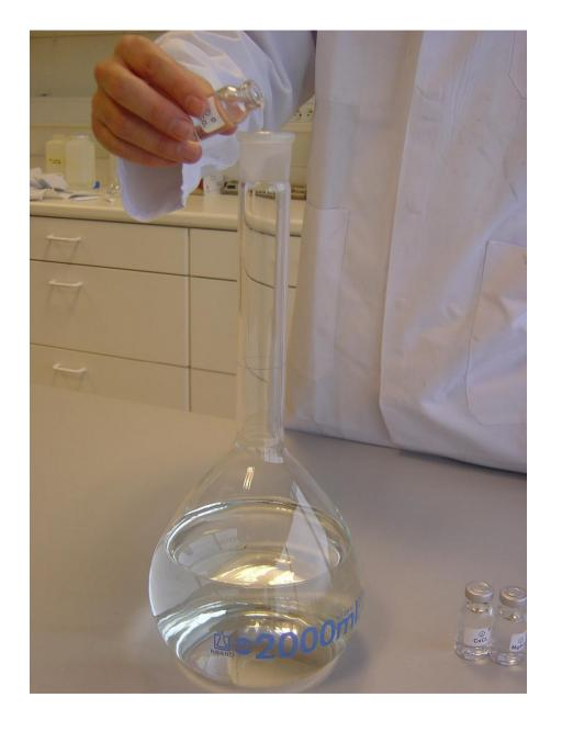
POUR THE 4 VIALS WITH CONCENTRATED SALT SOLUTIONS IN  $\pm$  1 LITER DISTILLED WATER, IN THE 2 LITER VOLUMETRIC FLASK
