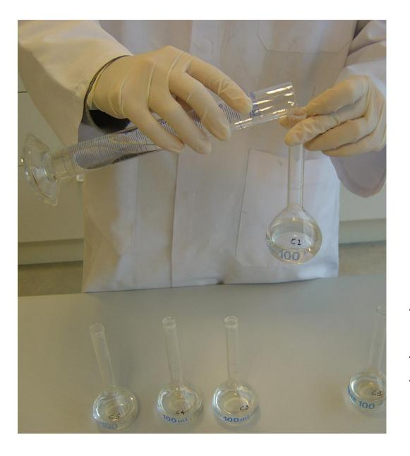
TRANSFER THE 50 ML EFFLUENT
